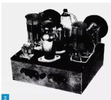
Fig. 1: For those who like to examine the theoretical circuit, this diagram will give them all the details they require. Note the alternative 'phone circuit. Fig. 2: A rear view of the assembled receiver showing the aerial series condenser located in an easily accessible spot. Fig. 3: Top of chassis component placement. Fig. 4: Under chassis wiring and component placement. Fig. 5: Plan view of the underside of the chassis, showing the exact location of parts and the associated wiring.
