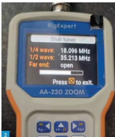
Fig. 1: The PL259 connector on the 75Ω coax. Fig. 2: Checking out the stub tuner. Fig. 3: Preparing the feedpoint to accept the loop. Fig. 4: One end of the loop connected temporarily during tune-up. Fig. 5: The loop installed ready for measurement. Fig. 6: Tuning too low. Fig. 7: Now resonant in band. Fig. 8: Possible loop configurations.
